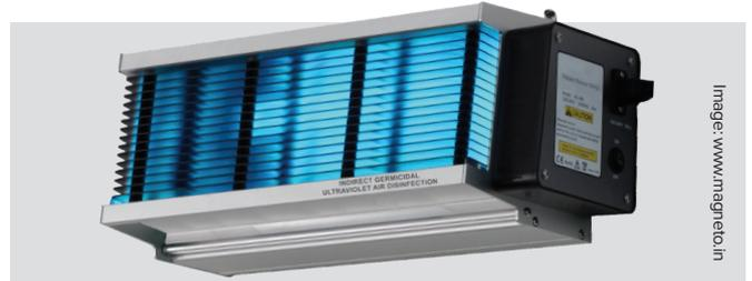
These devices mount on the wall and plug into a 230V power supply. They are normally passive and don't have fans. They rely on good mixing of the room air to ensure that all air has time in the irradiated zone. They become less effective at high air change rates due to the reduced exposure time.
